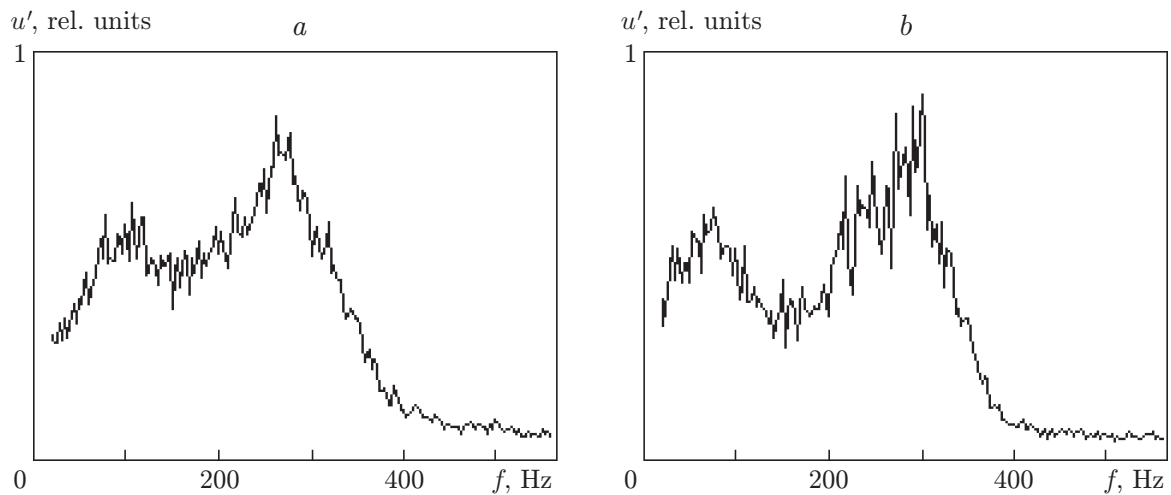
Fig. 2. Spectra of disturbances: (a) h = 3.0 mm and x/h = 18.7 ; (b) h = 2.9 mm and x/h = 20.0 .
